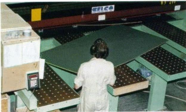
**Cutlists for panels machined on this Selco panel saw are downloaded directly from the front office.**
