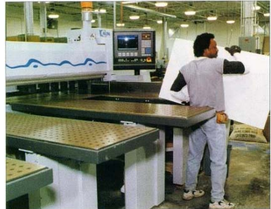
At the head of the manufacturing scheme at Lannon Miliwork is a new Holzma HPP1 1 GNC panel saw which generates a barcode label with all manufacturing information included.
